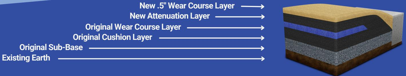
Both solutions include complete removal of the perimeter (4" to 12") allowing the new surface to properly bond the edge and taper up from the curb/sidewalk to maintain an ADA accessible access.
