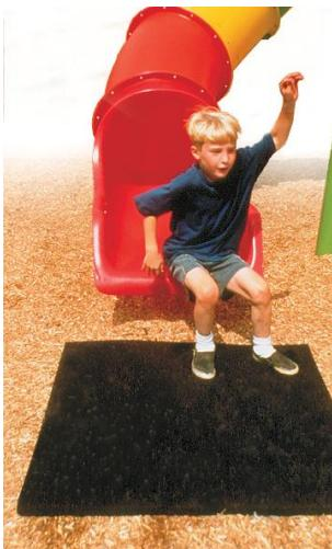
Designed with a beveled edge on all four sides for accessibility, these black rubber mats provide extra protection in hard use areas such as under swings and at slide exits. To prevent displacement of the Fibar in high-use areas and reduce maintenance, FibarMat wear mats must be installed under all swings, tire swings, slide exits, and all other wear areas including sliding poles. These will help to ensure compliance with the intent of the Americans with Disabilities Act.
