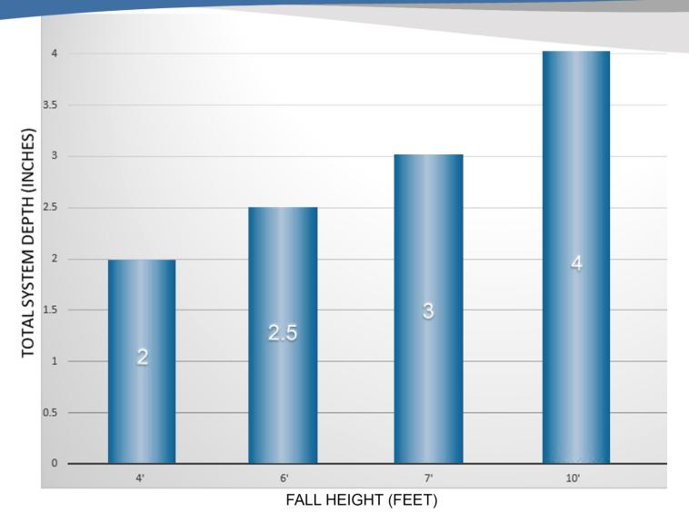
CHART REPRESENTS THE TOTAL (SBR CUSHION & TPV WEAR COURSE) SYSTEM DEPTH EXAMPLE: 2.0" SYSTEM CONSISTS OF 1.5" SBR CUSHION LAYER AND 1/2" TPV WEAR COURSE
