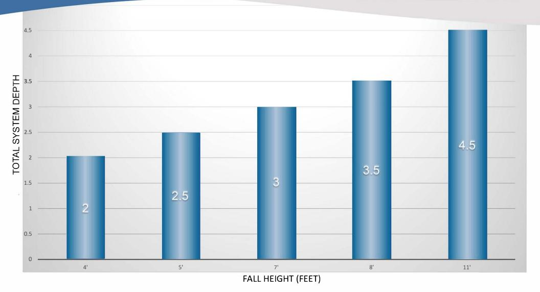
CHART REPRESENTS THE TOTAL (SBR CUSHION & TURF) SYSTEM DEPTH EXAMPLE: 2.5" SYSTEM CONSISTS OF 2" SBR CUSHION LAYER AND APPROX. 1" TURF with .5" infill
